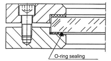
Bauform 120-V (O-ring sealing)
