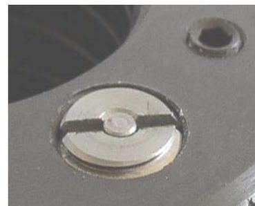
Picture shows pressure indicator visible up to 1. mark.
